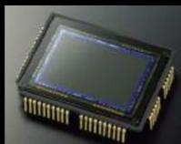
Sensor CCD (*Charge -Coupled Device*)
